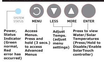
**Main Screen:** In normal operating mode the main screen displays the current WATER temperature, TARGET Temperature and if SOLAR HEAT, NOCTURNAL COOLING or FREEZE is ON or OFF. Press the Enter button to view the current Water and Solar temperatures. If no menu activity is detected after two minutes, the main screen is displayed.
